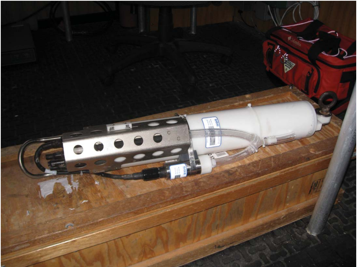
Figure 11: R/V BAY HYDRO II's SeaBird 19plus CTD.
