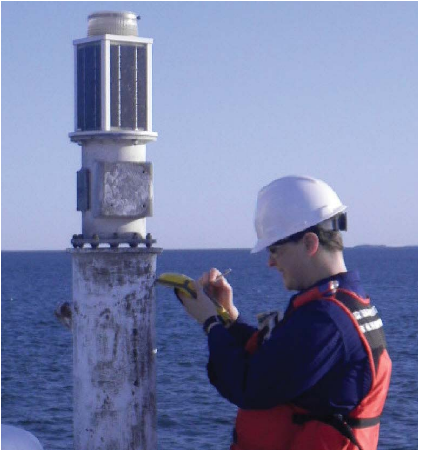
Figure 24: Shoreline verification of the features with a Trimble GeoXH.
