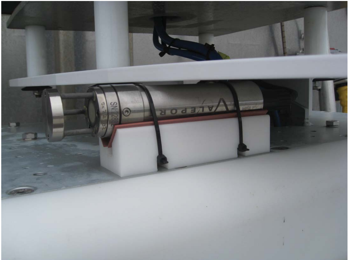
Figure 13: Valeport MiniSVP mounted to the MBES case.
