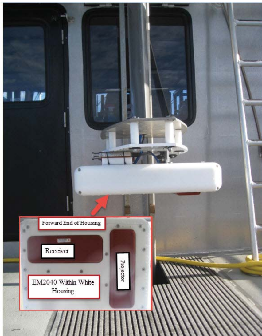
Figure 3: Kongsberg EM2040 housing and sonar, in the retracted position.
