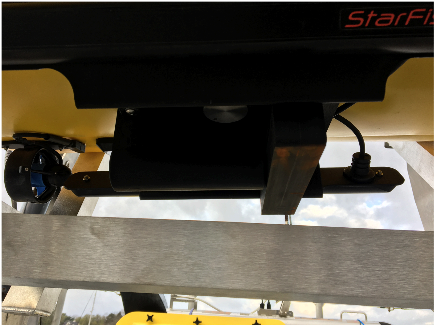
Figure 2: PicoMB-120SF mounted on ASV 008.
