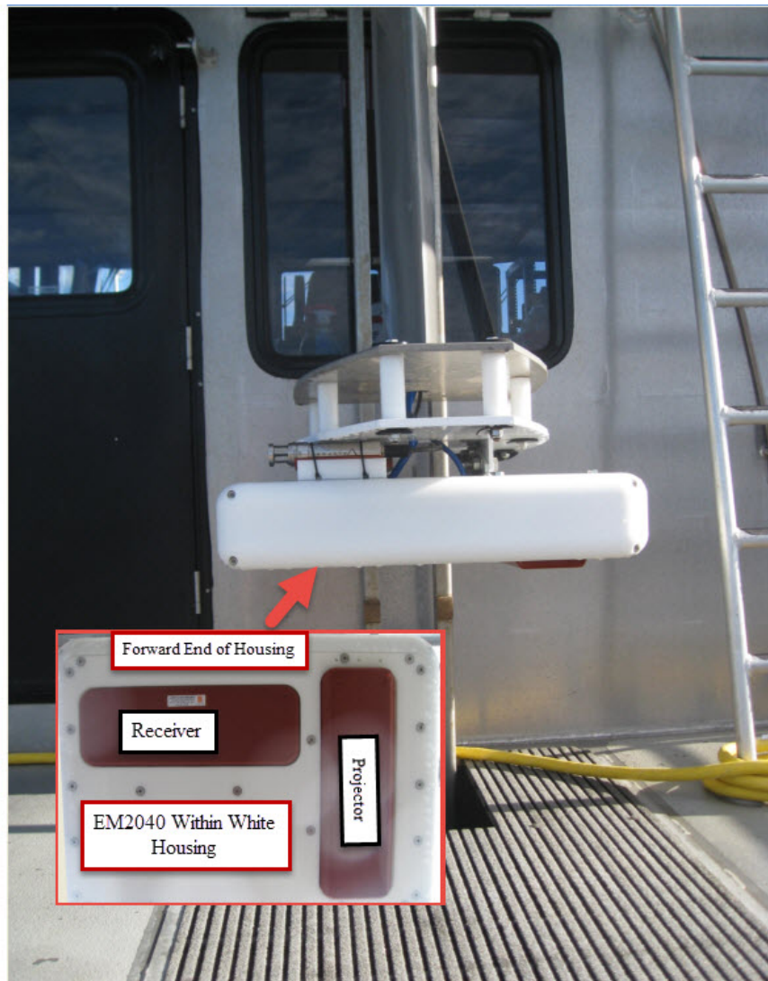
Figure 2: Kongsberg EM2040 housing and sonar, in the retracted position.
