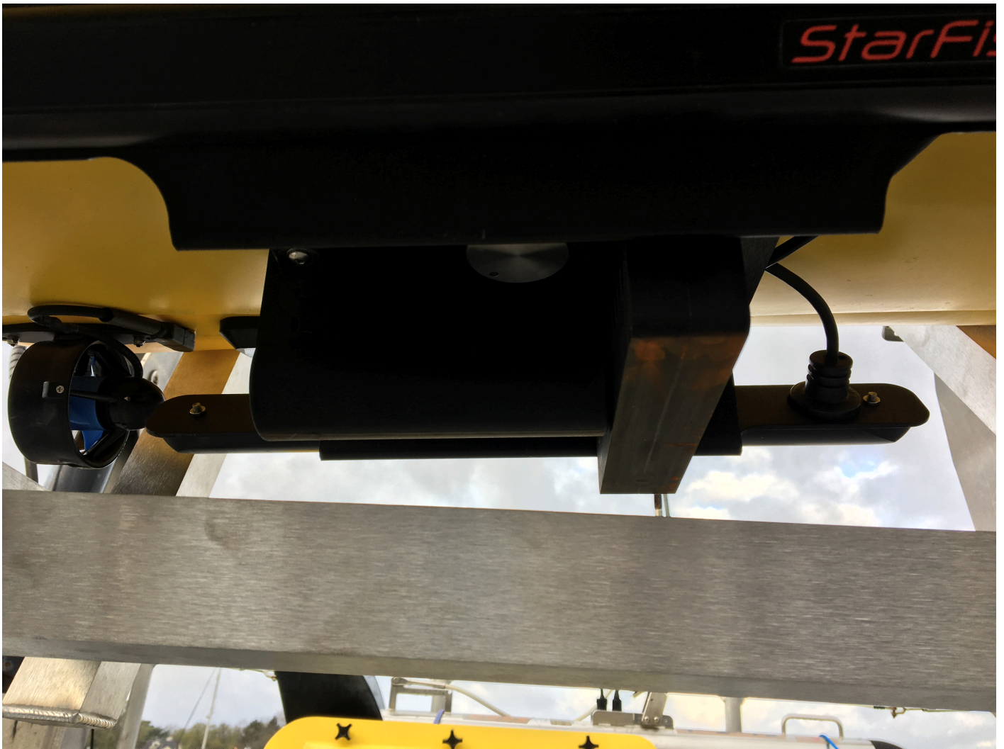
Figure 5: PicoMB-120SF mounted on ASV 008.
