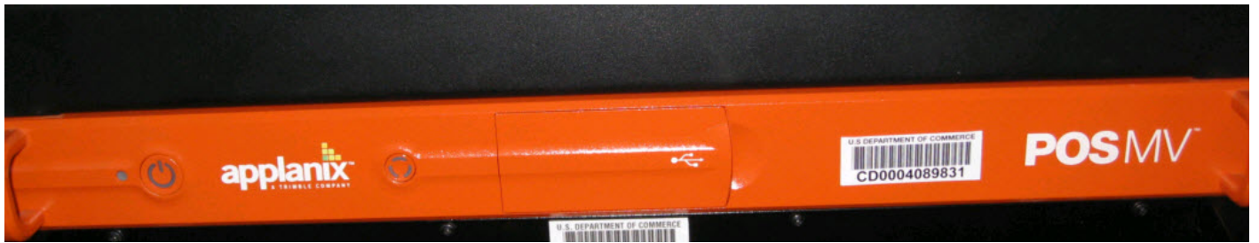
Figure 6: POS/MV computing system unit (orange) rack mounted aboard R/V BAY HYDRO II.
