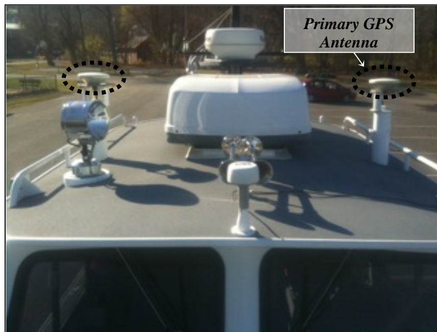
Figure 2: POS/MV Antenna Installation
