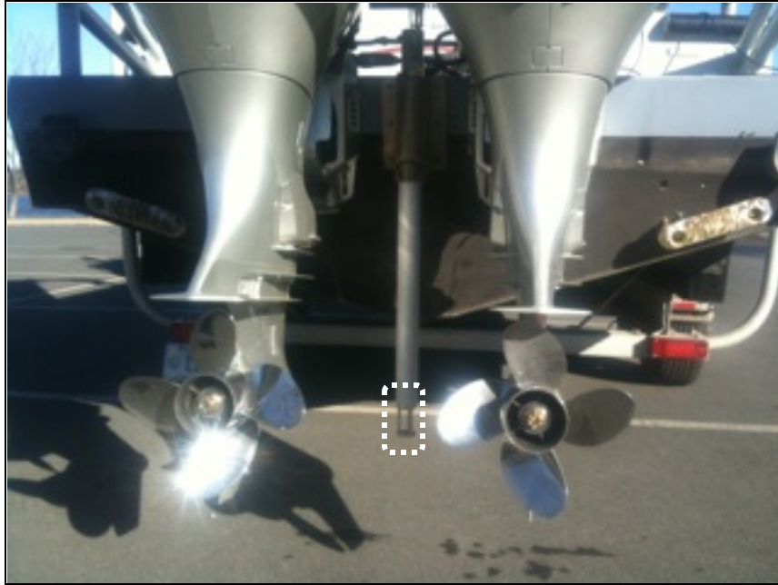
Figure 4: Surface Sound Speed Digibar Installation
