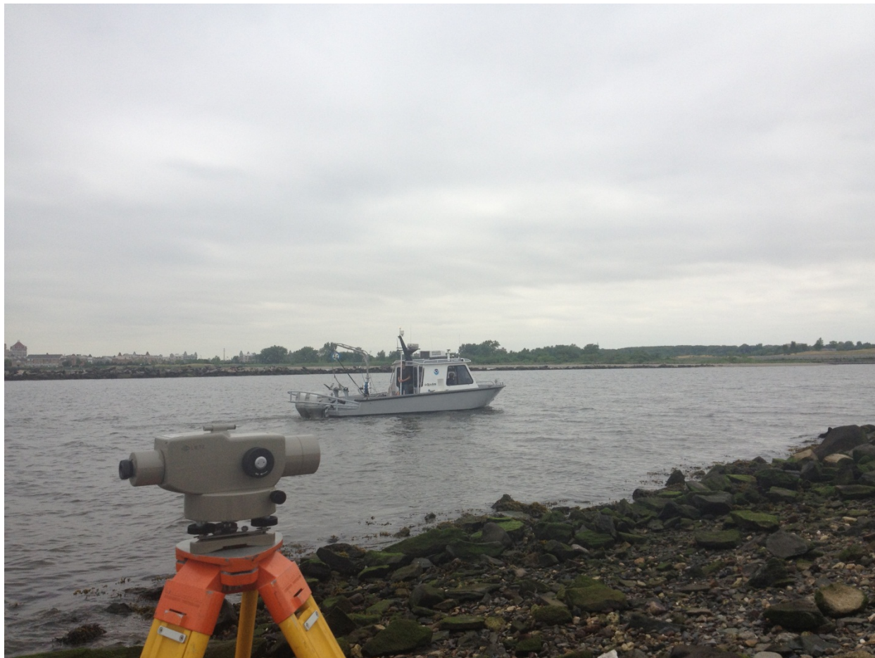
Figure 11: Dynamic Draft Optical Level Setup
