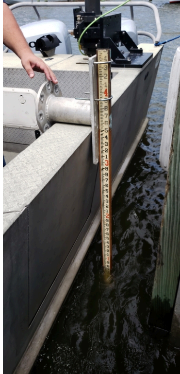
Figure 12: Static Draft Gauge made from tide staff
