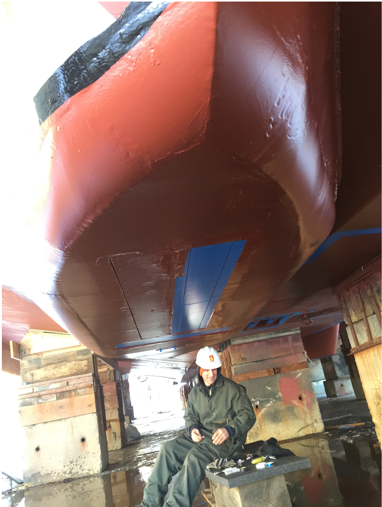
Figure 4: The EM710 system mounted on the hull of R352, shown during installation in 2015.
