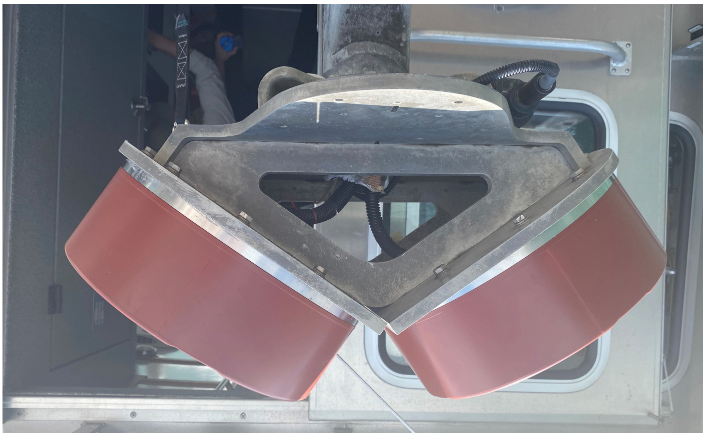
Figure 2: Kongsberg EM2040C dual-head sonar on the R/V Chinook pole mount
