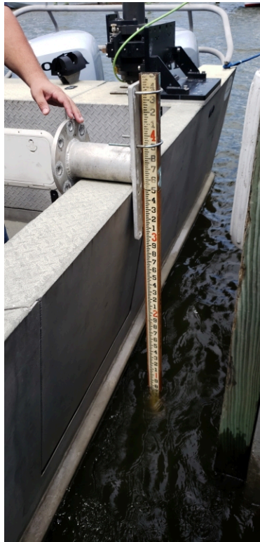
Figure 14: Static Draft Gauge made from tide staff
