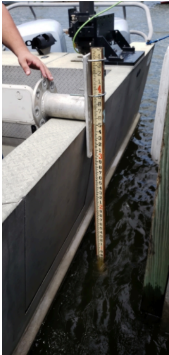
Figure 11: Static Draft Gauge made from tide staff
