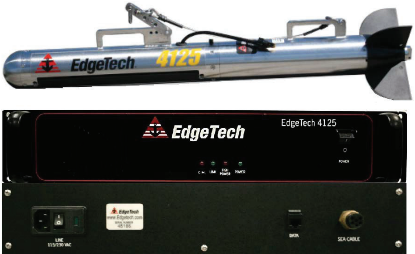
Figure 3: EdgeTech 4125 towfish and rack mount processing unit.
