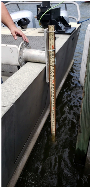
Figure 14: Static Draft Gauge made from tide staff
