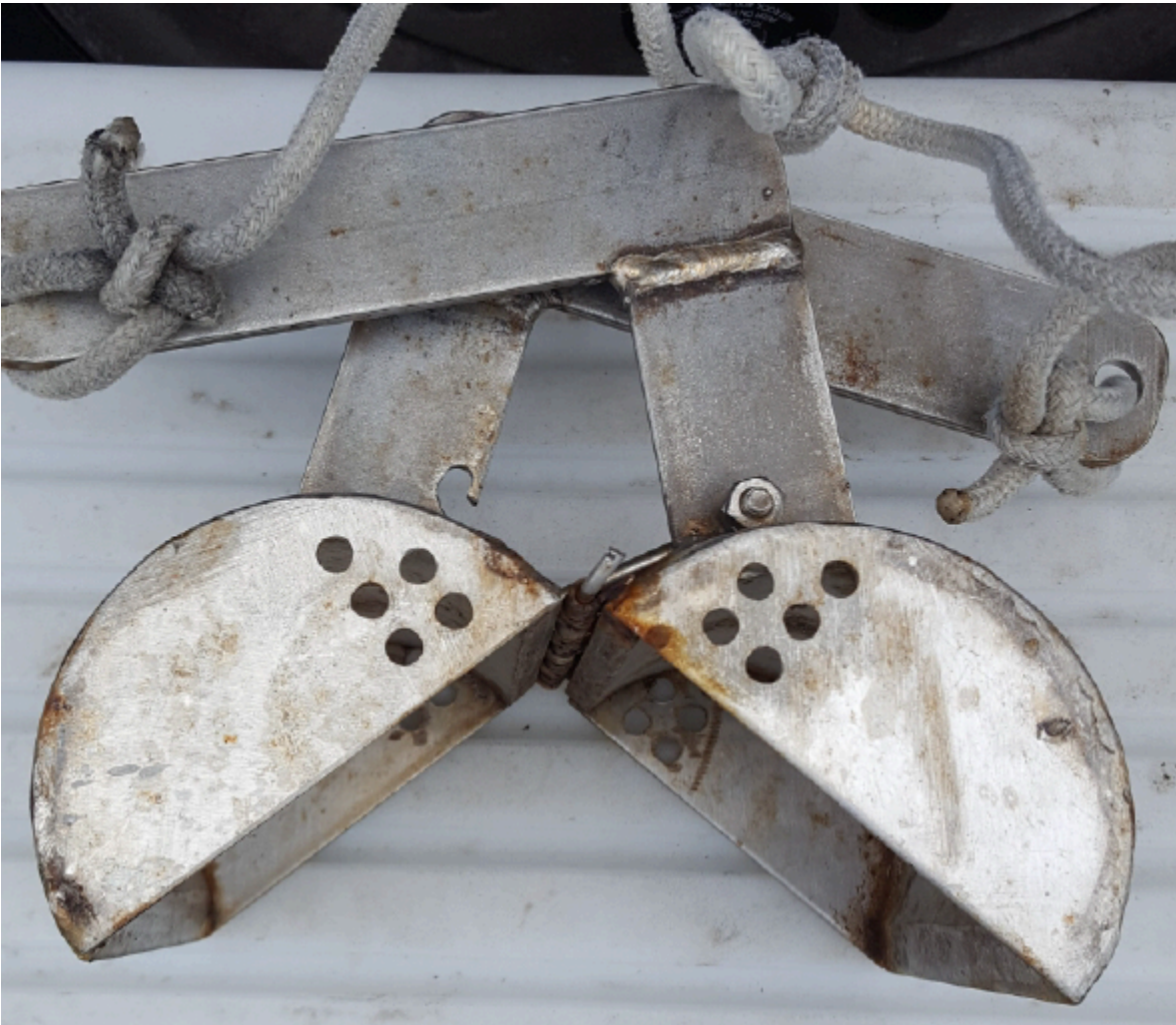
Figure 7: Clam Shell-style, 4 inch bottom grabber
