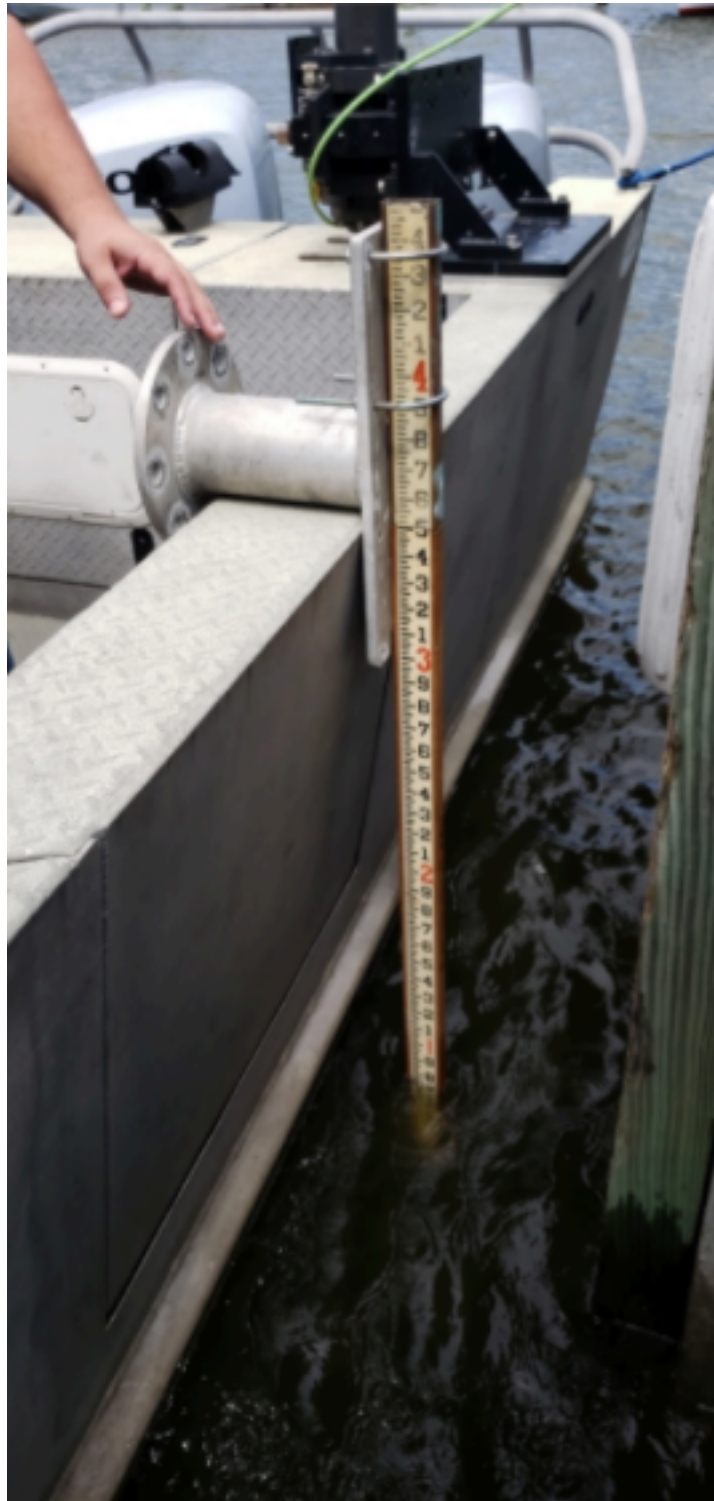
Figure 15: Static Draft Gauge made from tide staff
