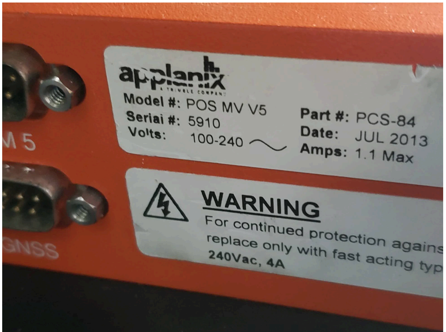
Figure 4: POS MV-320 V-5 GNSS-aided inertial navigation system
