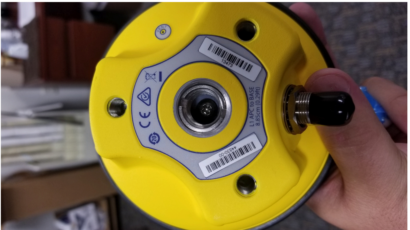
Figure 6: Primary Antenna Trimble GA830
