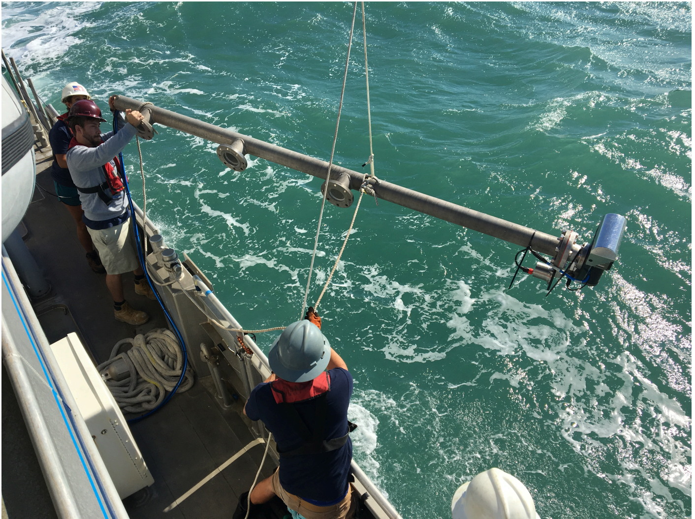
Figure 3: T20P Sonar installed on survey arm being lowered into place.
