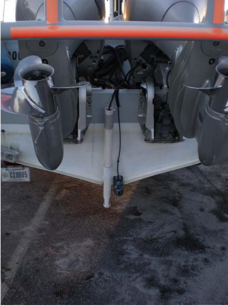
A problem with this configuration is the tendency for air bubbles and large debris to become trapped in the PVC tube, leading to large errors in the sound velocity. This in turn causes the multibeam to incorrectly steer the incoming pings, seen as large “frowns” in the bathymetry. Data exhibiting this problem are noted, and data are re-acquired over the problem areas.
