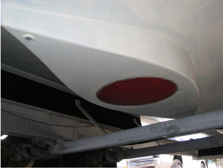
Figure 1: Hull-mounted Simrad EM 3002 transducer.
