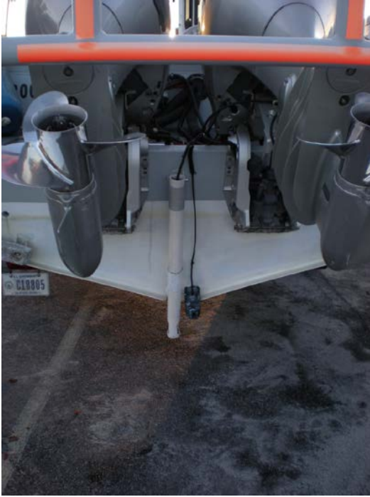
Figure 2: S3003 Digibar and AML mount with protective PVC sheath.
