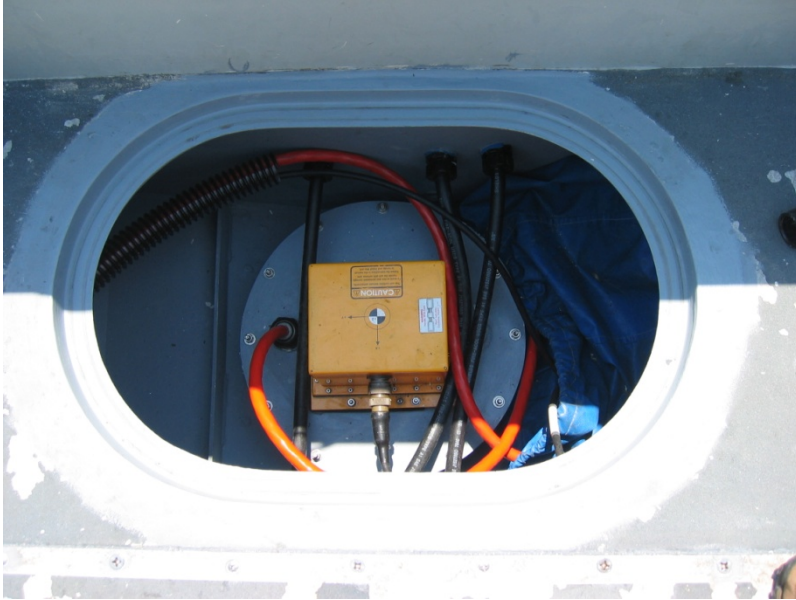
Figure 4: IMU mounted in hatch directly above the multibeam transducer.
