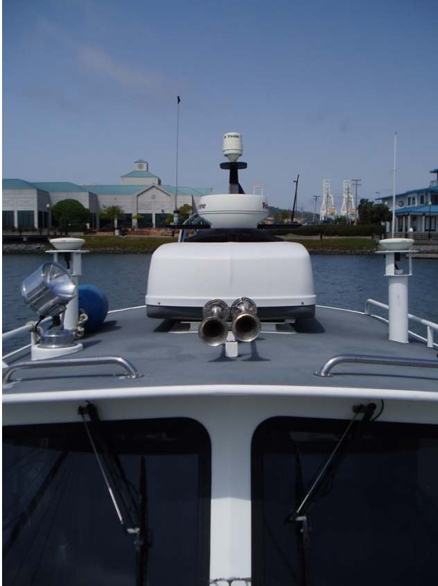
Figure 5: View of top of house on Launch S3003. Center GPS antenna is used by Trimble DSM 132 receiver, and two lower antennae are used by the POS/MV.
