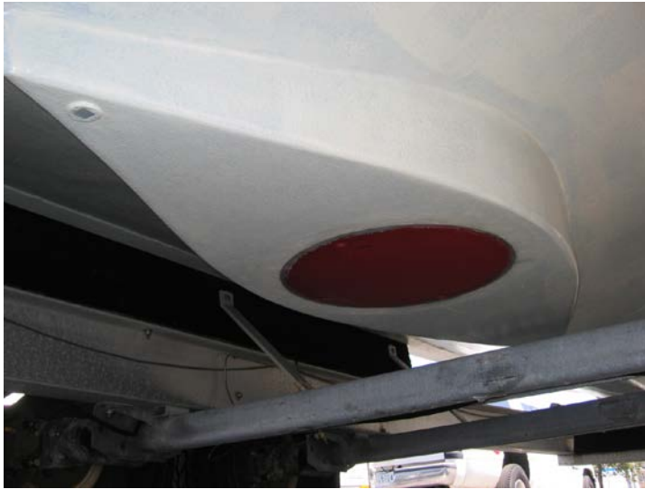
Figure 1: Hull-mounted Simrad EM 3000 transducer.
