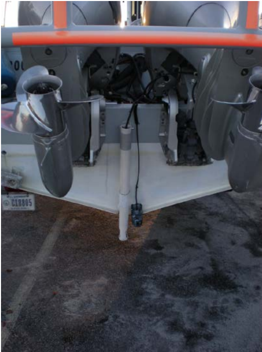
Figure 2: S3003 Digibar mount and protective PVC sheath.
