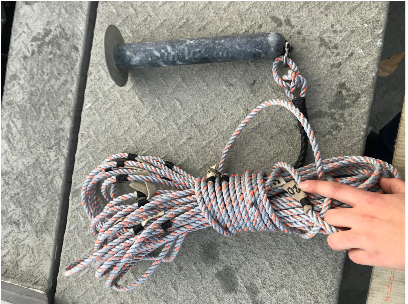
Figure 5: NRT-3's lead line, good for depths up 20 meters.
