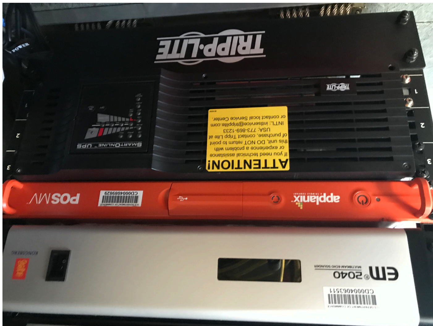
Figure 8: POS MV installed in the server rack on S3006.
