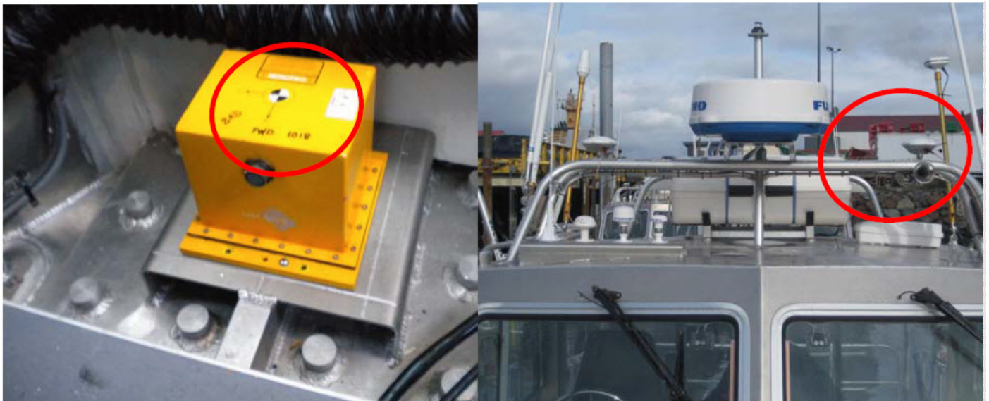
Figure 38: Vessel Reference Point (Top of POS MV IMU) & Primary GNSS Antenna (port side).
