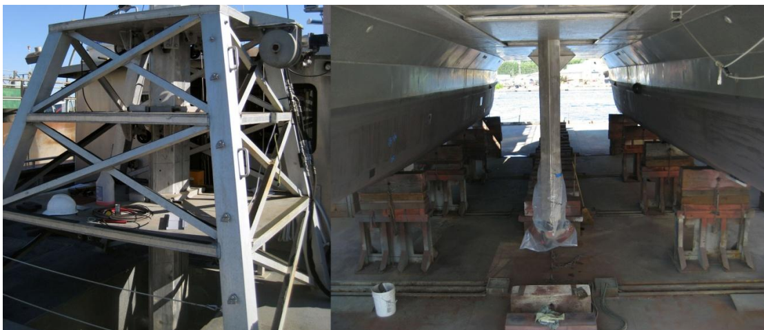
Figure 3. Derrick mounted on aft deck (left) and dual heads shown on retractable pole (right).
