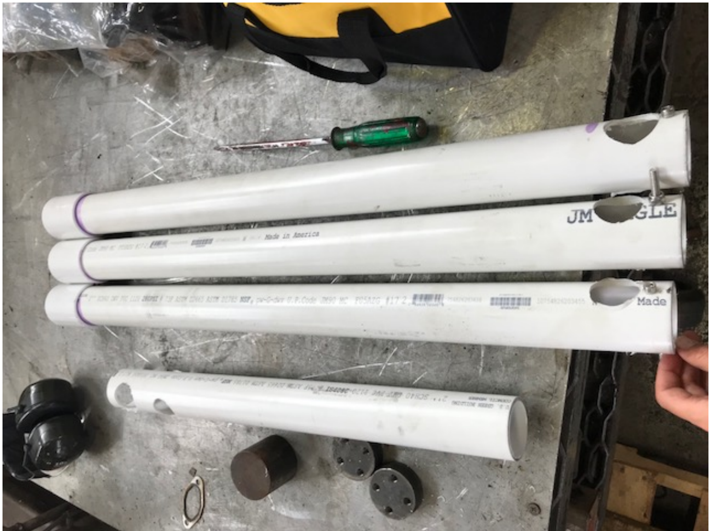
Figure 13: The PVC poles that are mounted inside a bracket on the transom that holds the AML sensor while surveying. The hole in the bottom of the tube allows for water flow over the sensor.
