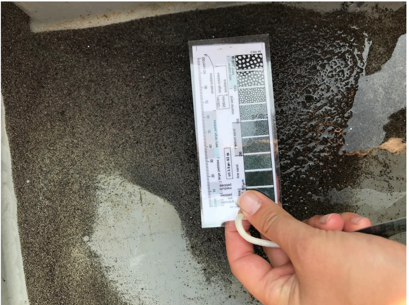
Figure 27: An example of the bottom sample from Portland, OR area.
