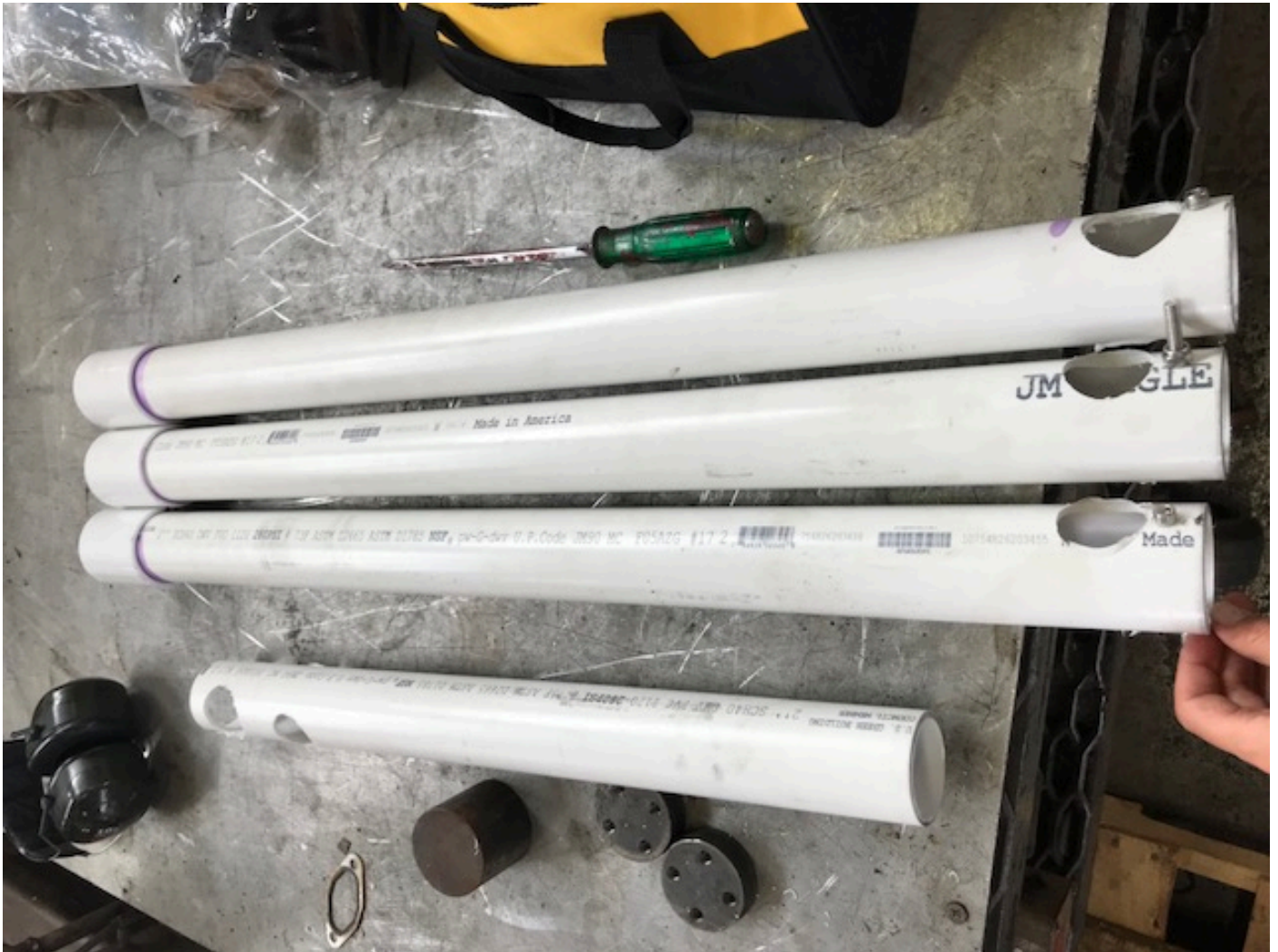
Figure 12: The PVC poles that are mounted inside a bracket on the transom that holds the AML sensor while surveying. The hole in the bottom of the tube allows for water flow over the sensor.
