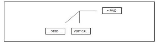
Top Center of IMU is origin of Hypack Coordinate System
