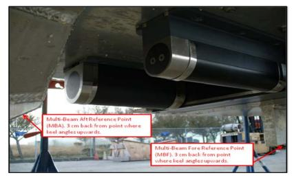
A point on the Multi-Beam transducer (MB) was measured directly this survey. The measured point was at the center of the bottom of the transducer. No mark was left to indicate the measured point.
