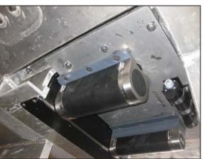
Figure 6: Reson 7125 SV transducer arrays
