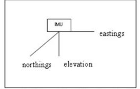
Bottom Center of IMU is origin of Westlake Coordinate System
