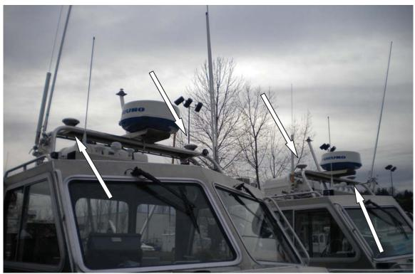
Figure 10: POS GNSS Antennas
