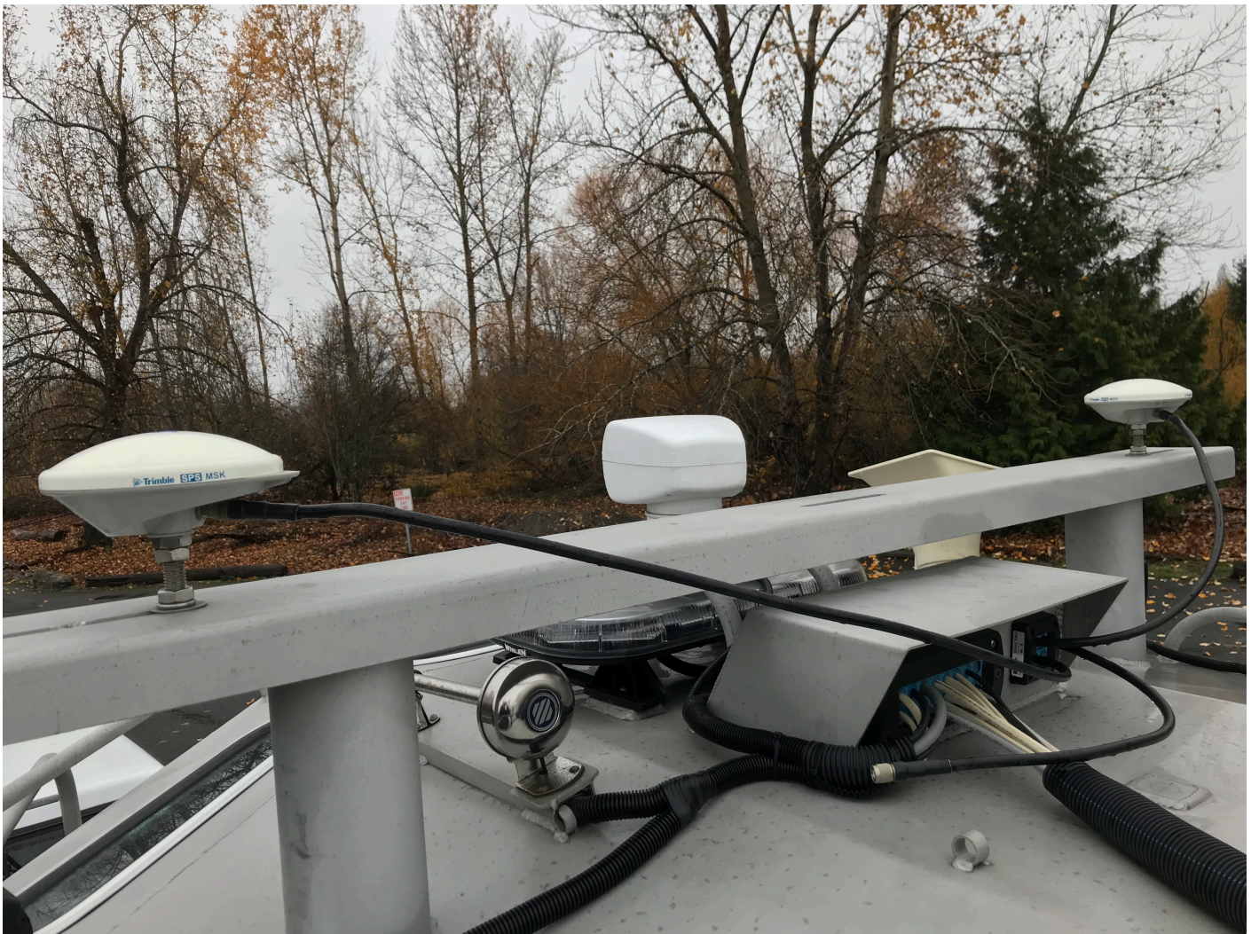
Figure 6: POS MV V5 system components: IMU, POS Computer System, and two GNSS antennas.
