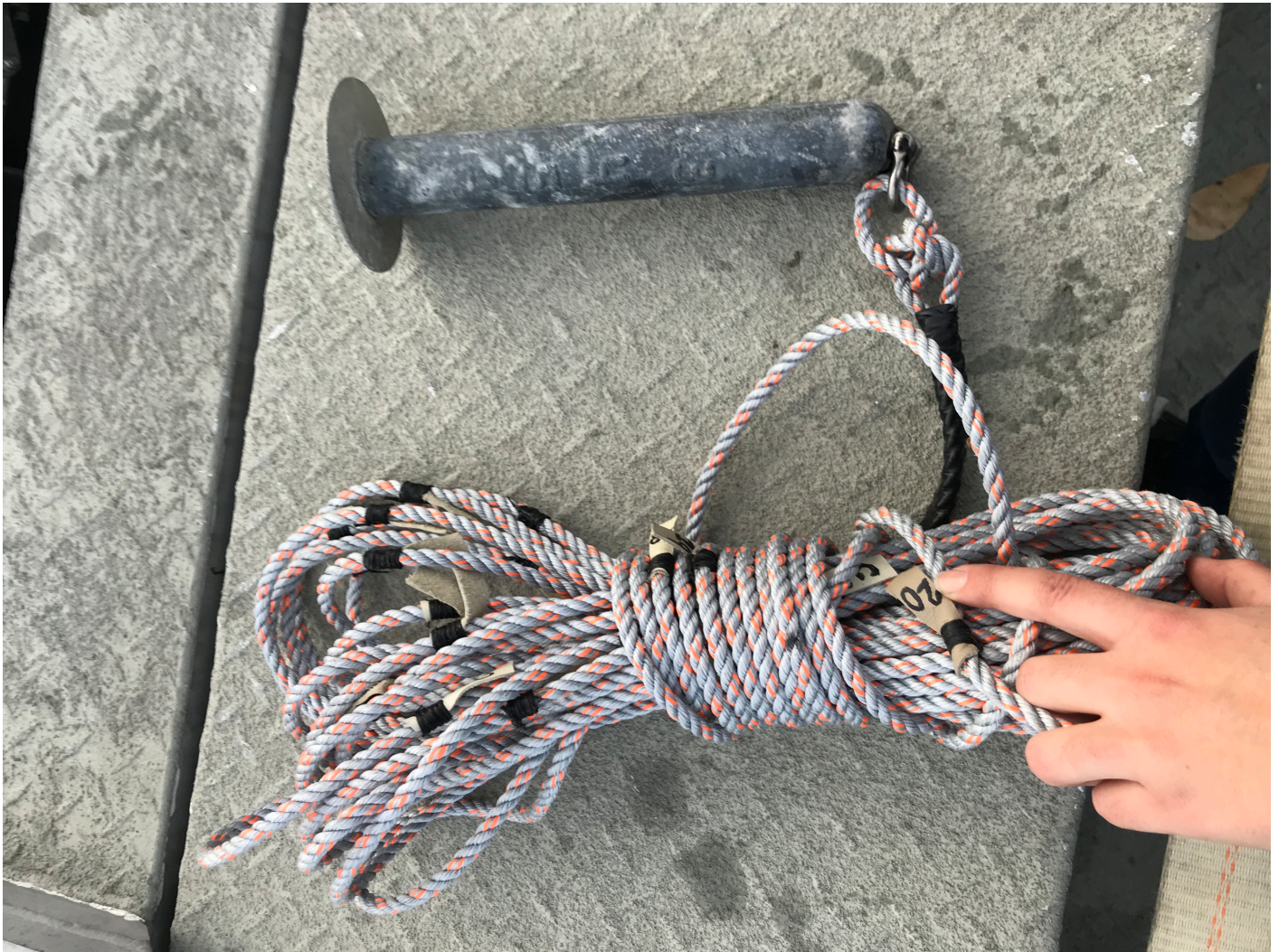
Figure 5: NRT-3's lead line, good for depths up to 20 meters.
