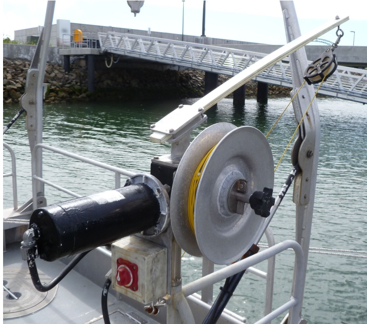
Figure 21: The 24v electric SV winch (note the knob at the side of the spool which controls deployment speed)
