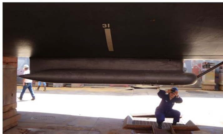
Figure 6: Kongsberg EM 710 sonar transducer housing on Rainier (S221)
