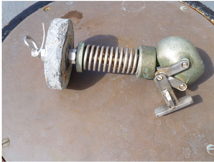
Figure 17: The KAHLISCO No. 214WA110 Mud Snapper, a clam shell style bottom sampler.
