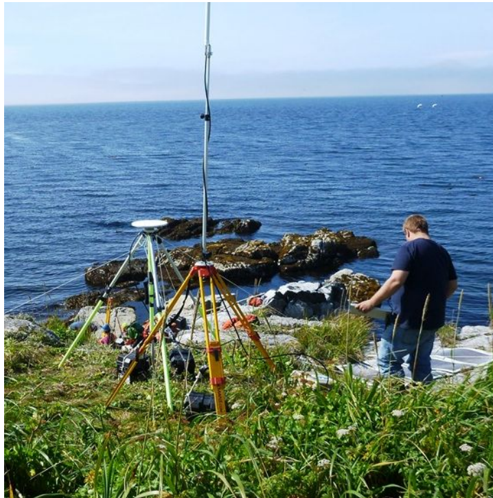
Figure 16: An example of a horizontal control base station consisting of a fixed height GPS tripod, a UHF transmission antenna and a NetR9 receiver with associated batteries and solar panels.
