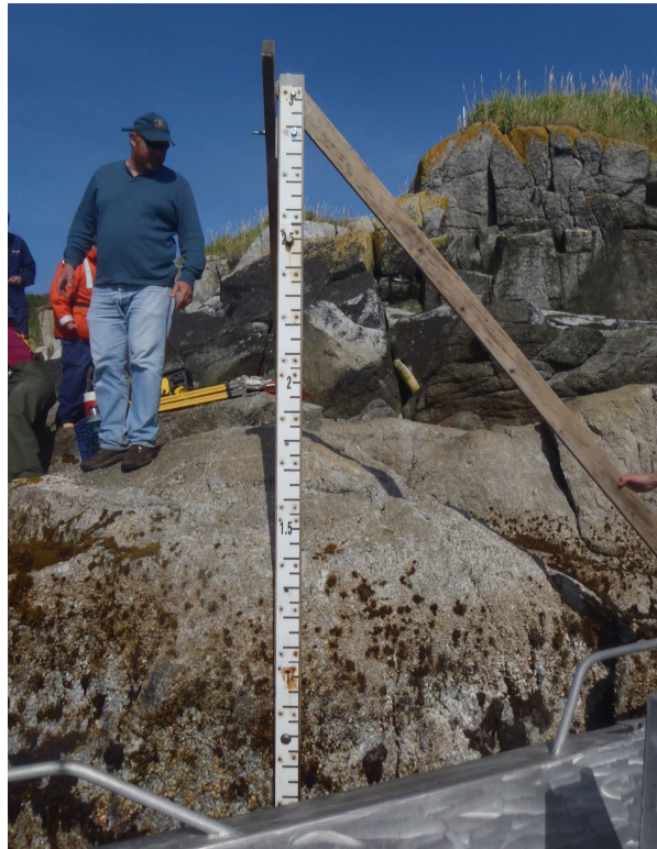
Figure 23: An example of a typical Rainier tide staff.
