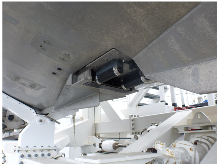
Figure 8: Reson 7125 mounted on survey launch 2801
