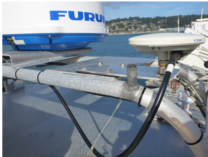
Figure 9: The aluminum extension bracket used to increase antenna separation of launches 2801 and 2802.
