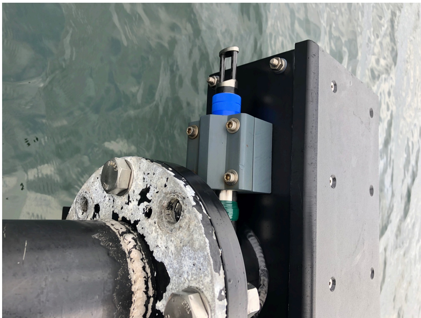
Figure 5: AML Micro•X installed on USM with a R2Sonic 2024
