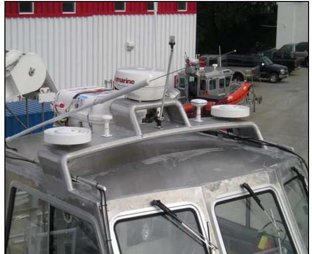
Figure 6: POS/MV antennas mounted on 1010 (side view)
