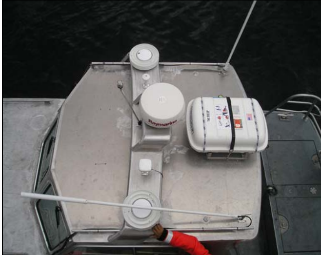
Figure 5: POS/MV antennas mounted on 1018 (top view)
