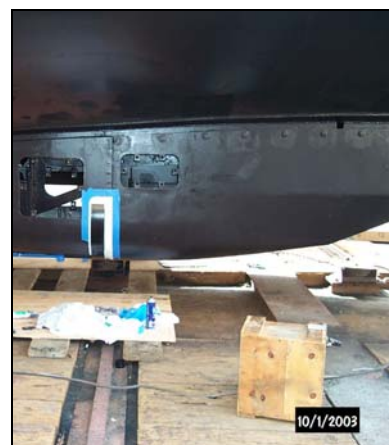
Figure 2: RESON SeaBat 8111ER MBES on FAIRWEATHER
