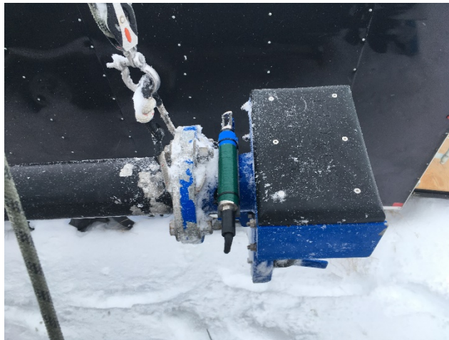
Figure 4: AML Micro•X Sensor Mobilized on an R2Sonic 2022
