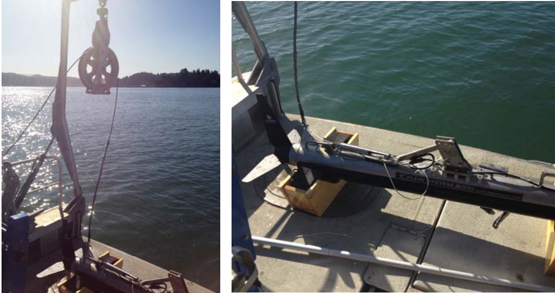
Figure 8: Launch-Towed Klein 5000 Side Scan Sonar
