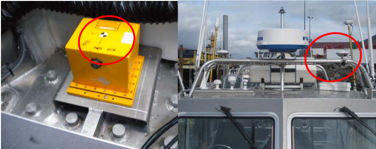
Figure 17: Vessel Reference Point (Top of POS MV IMU) & Primary GNSS Antenna (port side).
