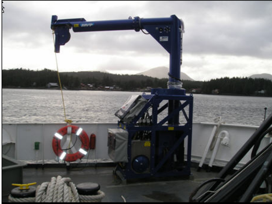
Figure 14: Fairweather's MVP200 sound velocity system
