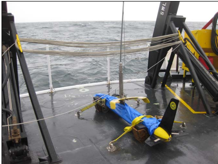
Figure 9: Towed Klein 5000 Side Scan Sonar on Fairweather
