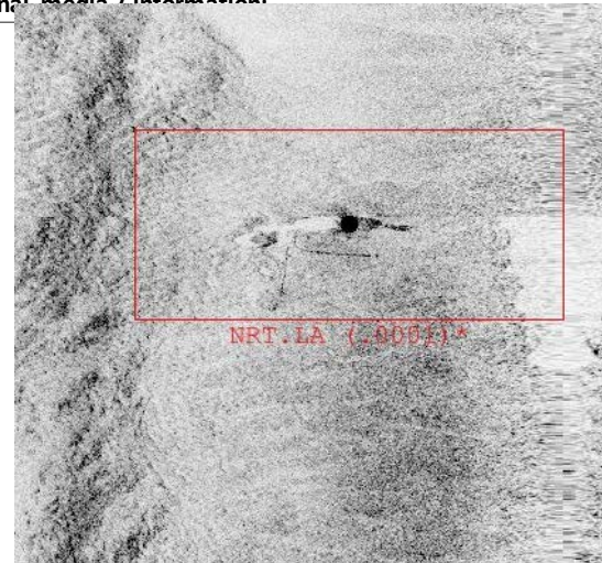
SSS imagery showing contact which rises ~4 m above the sea floor.
