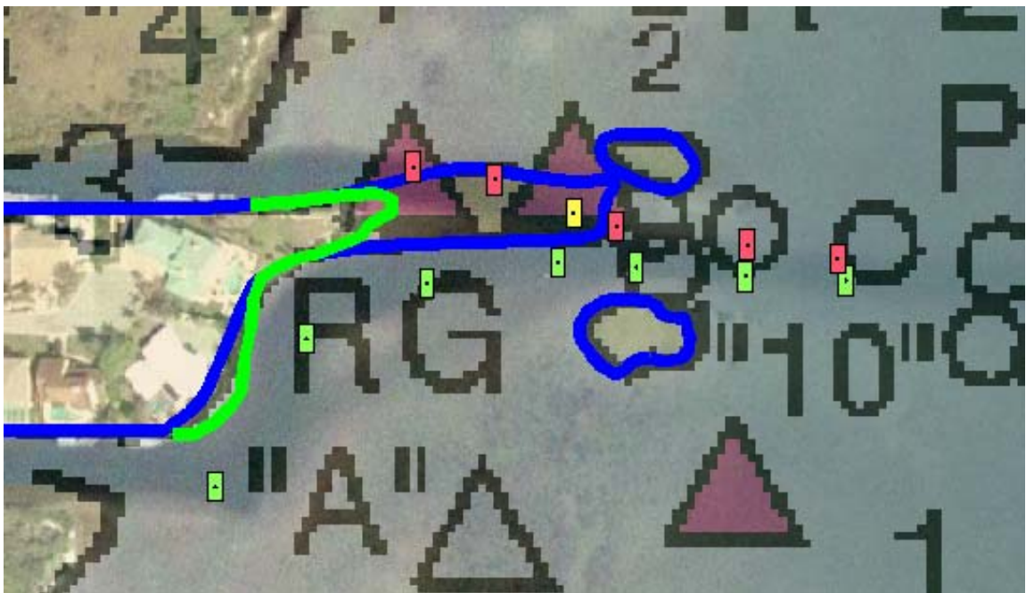
Figure 2: USGS 0.5-meter orthoimagery overlain with RNC 11481, surveyed beacons, existing shoreline (solid blue lines), and recommended shoreline modification (solid bright-green line)
