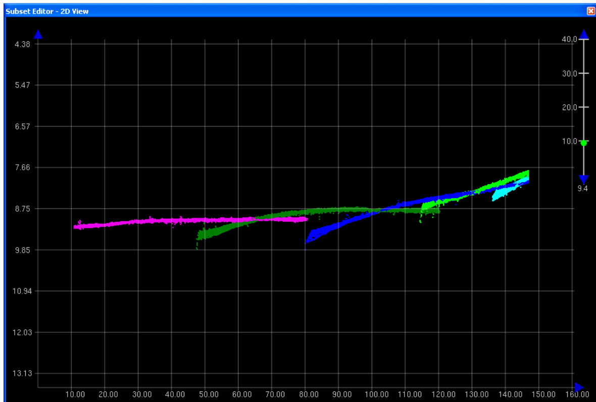
Figure 2: Example of sound speed artifacts in survey F00558
