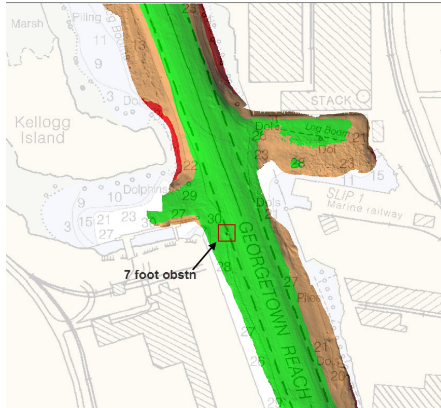
Figure 26: 7-foot high obstn on westerly edge of 30-foot channel.
