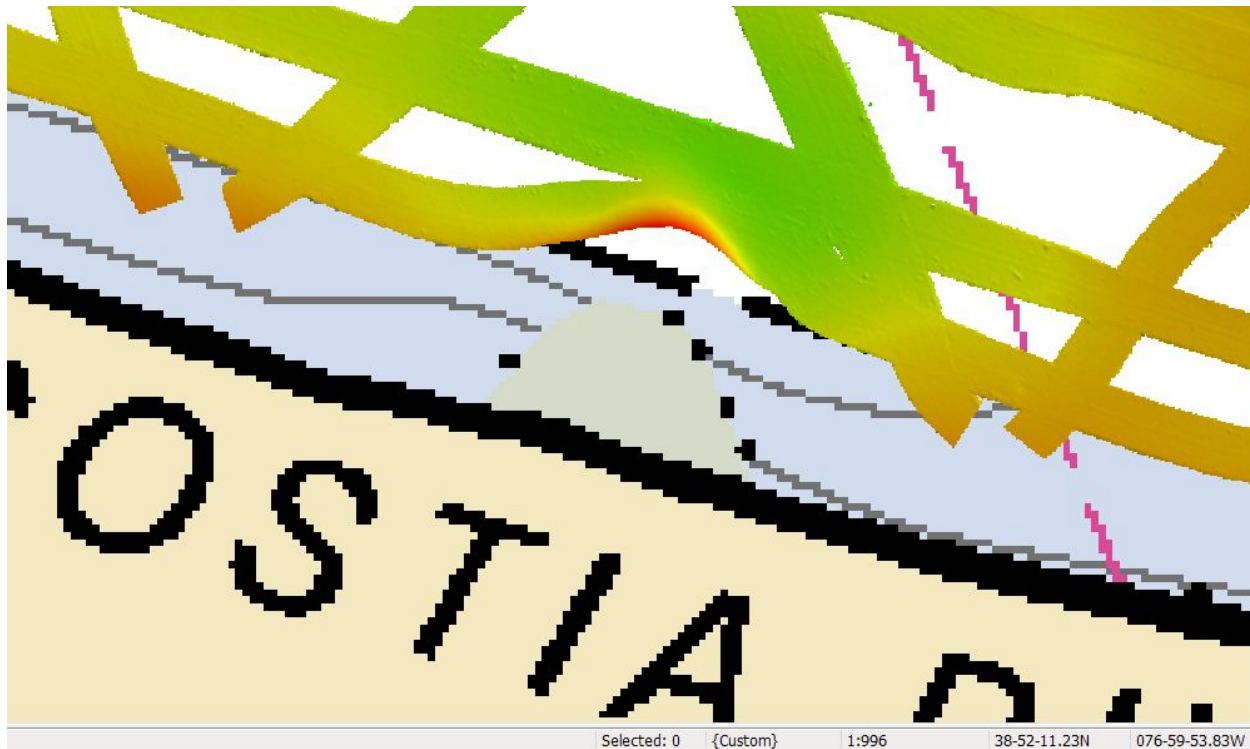
Figure 7: Chart 12289 shoal on the south side of the channel in the Anacostia River extends further into the channel than charted.
