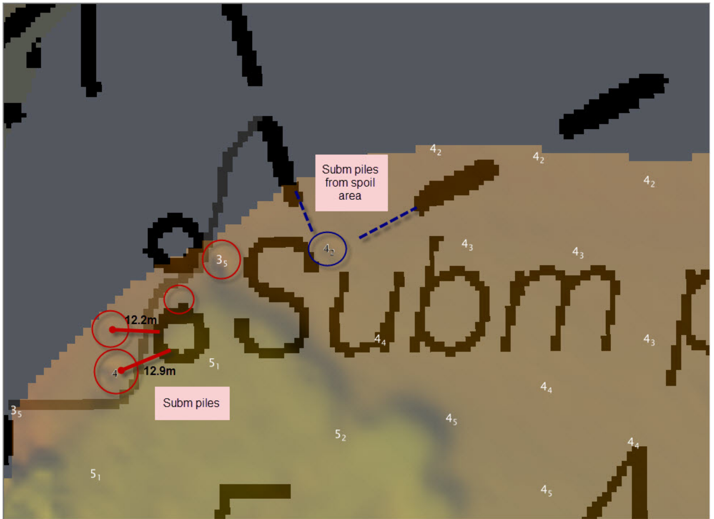
Figure 11: Disagreement between chart Submerged Pilings and surveyed soundings
