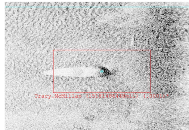
SSS imagery showing an obstruction, approx. 8.71 ft length, 3.00 ft width, and 4.65ft height.
