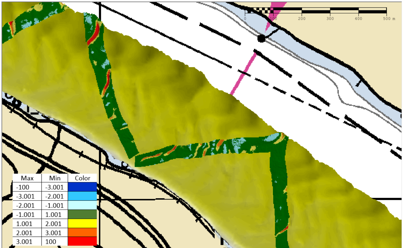
Figure 12: Less than 95% of nodes pass the crossline analysis of F00722 due to changing environmental conditions.
