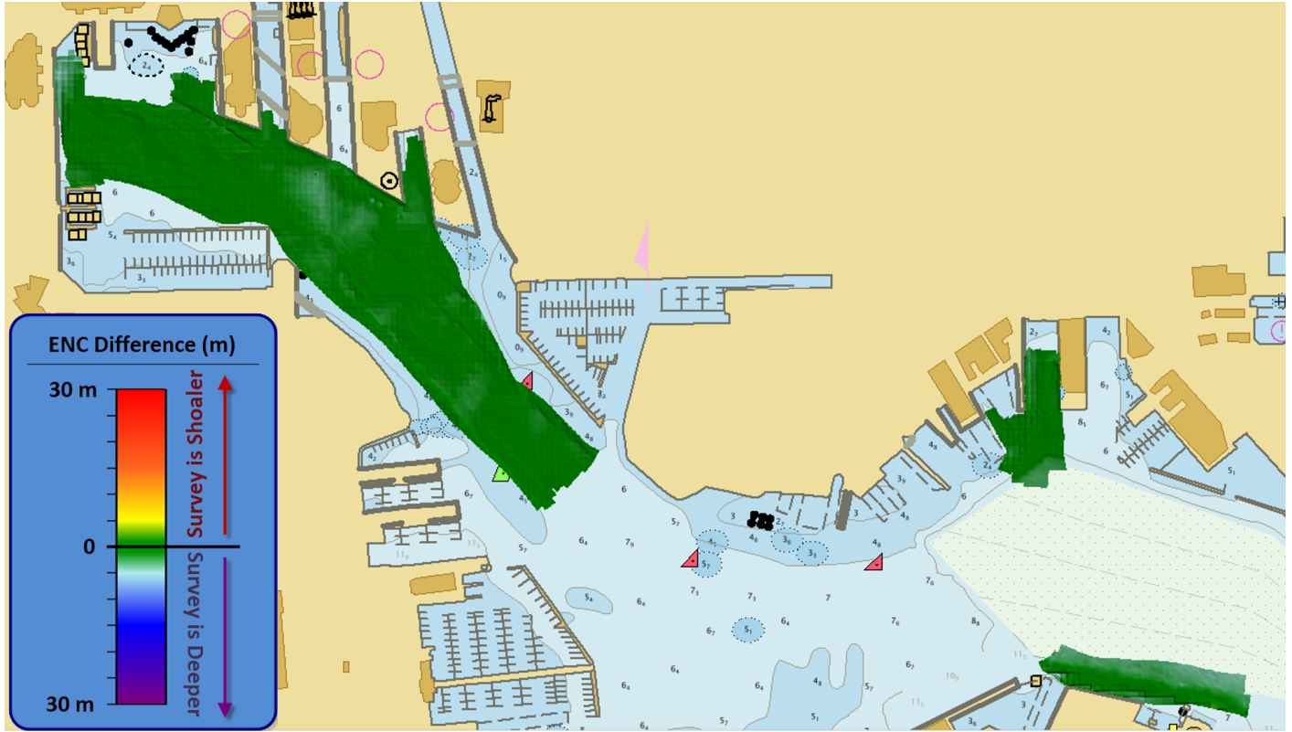
Figure 5: Difference surface between F00737 and interpolated TIN surface from ENC US5MD11M.
