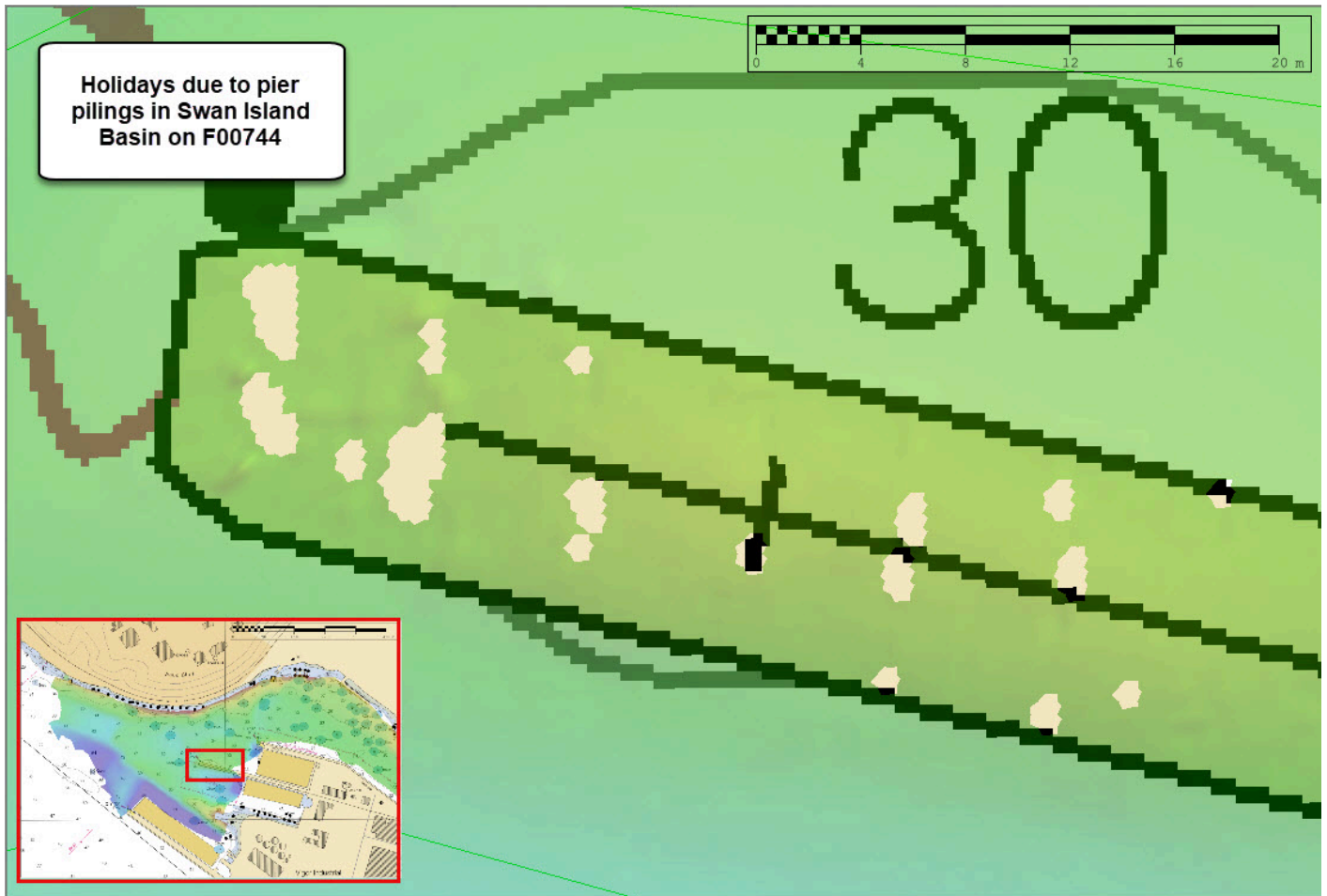
Figure 11: Holidays due to pier pilings in the Swan Island Basin. MBES data on pilings supporting an active pier were rejected from the data.
