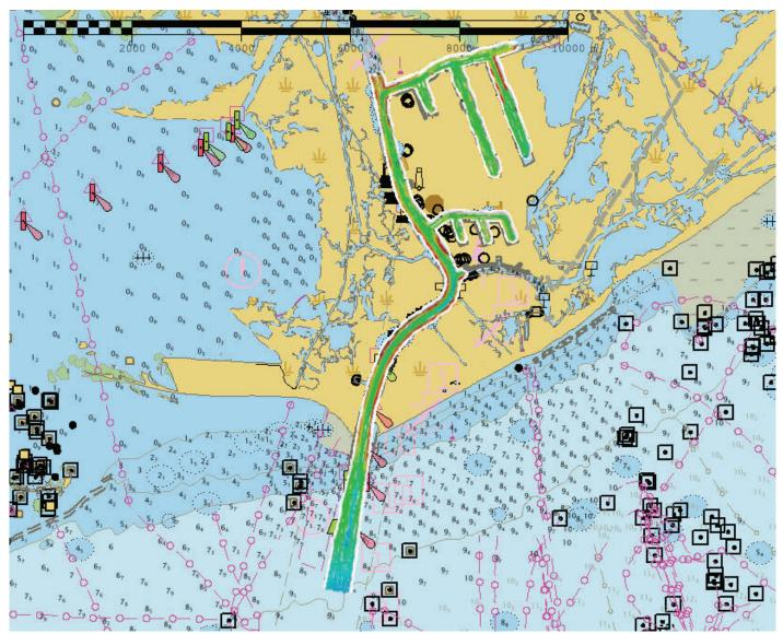
Figure 2: MBES and SSS coverage of Port Fourchon for F00774
