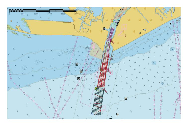
Figure 11: Tracklines symbolized by sound Velocity cast
