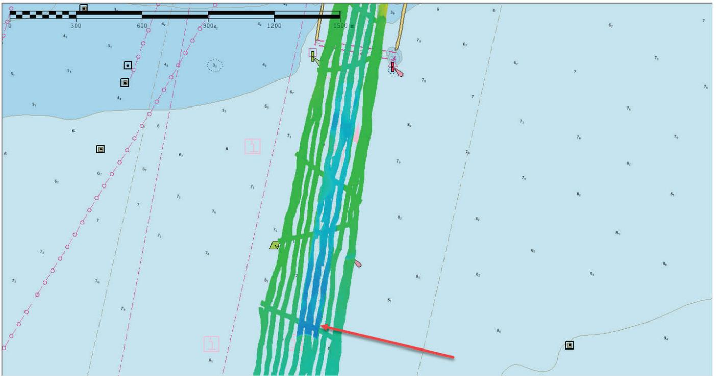
*Figure 17: Dredge area evident in the MB derived CUBE surface from F00774*
