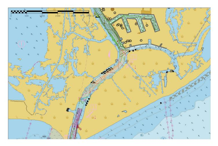
Figure 10: Tracklines symbolized by sound Velocity cast
