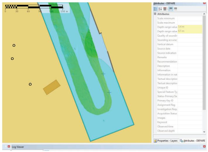
Figure 13: Depth Range of 5.4 to 9.1 meters, described on ENC US5LA26M
