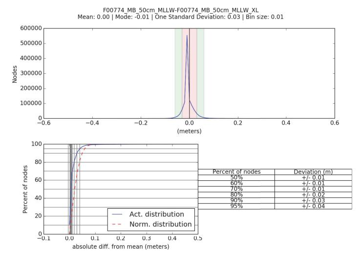
Figure 4: Distribution of the differences, between the crossline multibeam CUBE depth surface and the main scheme multibeam CUBE depth surface, about the mean
