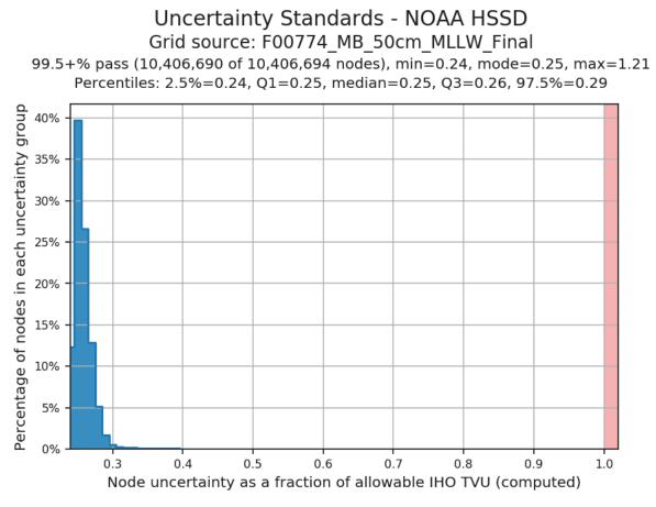
Figure 8: HSSD uncertainty standards for surface F00774\_MB\_50cm\_MLLW\_Final.csar
