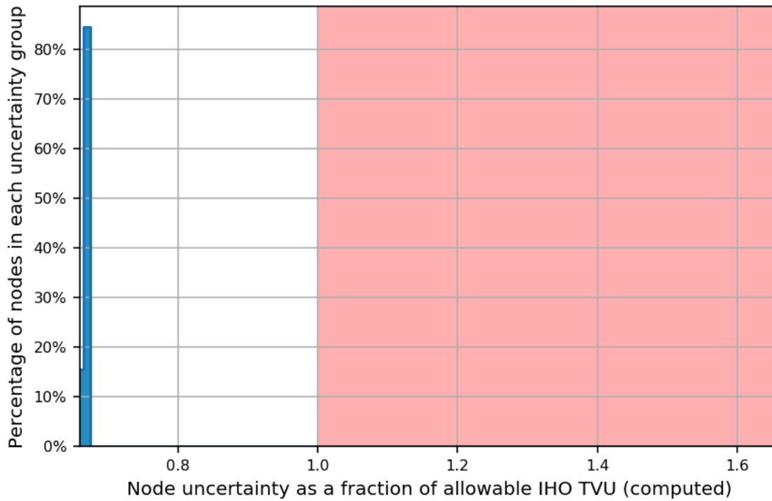
Figure 2: More than 99.5% of nodes in the finalized surface meet HSSD uncertainty requirements
