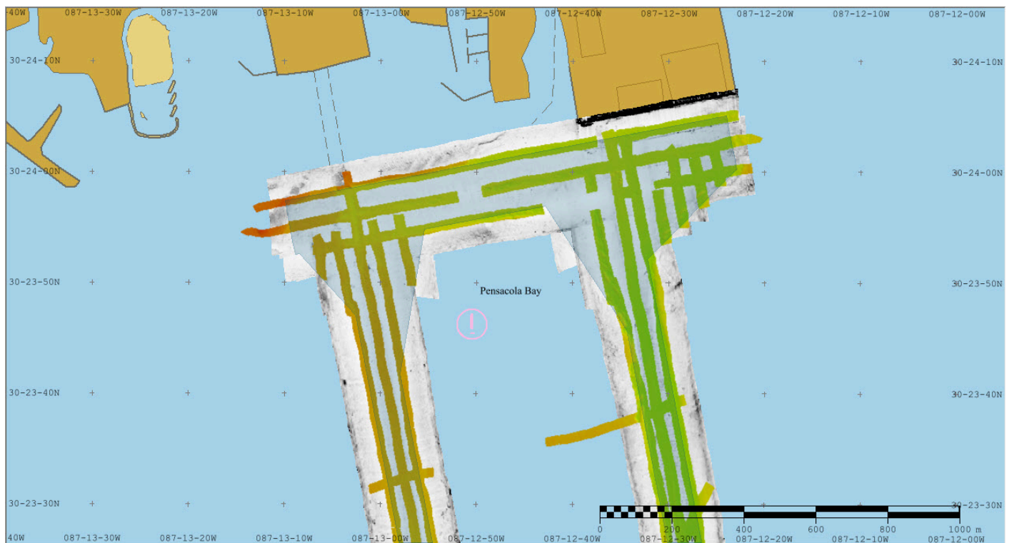
Figure 5: Gaps in concurrent multibeam coverage displayed over an associated 200% sidescan mosaic. A transparent survey limit shapefile is overlaid in order to depict the areas where object detection coverage was not achieved.
