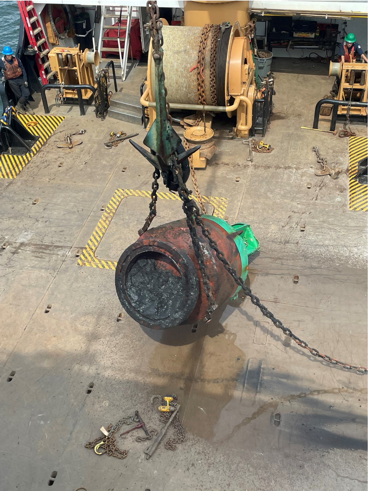
Figure 9: Buoy with chain being placed on deck after removal.
