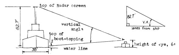
For a height of eye of 6' and a beam of 38', the resulting error is negligible; so that the following table considers no horisontal or vertical displacement.
