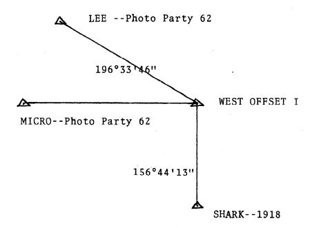
The geographic position of WEST OFFSET was computed using RK 409 "GEODETIC UTILITY PACKAGE", version 9/5/73.
