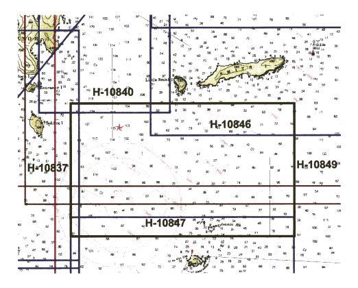
Soundings on these 1998 surveys were found to be in good agreement, generally matching within two or three meters. Final comparisons will be made at the Pacific Hydrographic Branch (PHB) after reduction to final vertical datum.
