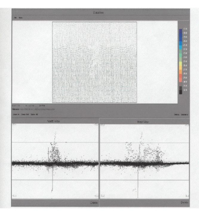
N.6 Two charted pipelines lie within the survey area. The positions of these pipelines were confirmed by side scan and multibeam sonar data. Positions along the pipelines were tagged and are listed in the sonar contact table. It is recommended that these pipeline locations be maintained as charted. Concur.
