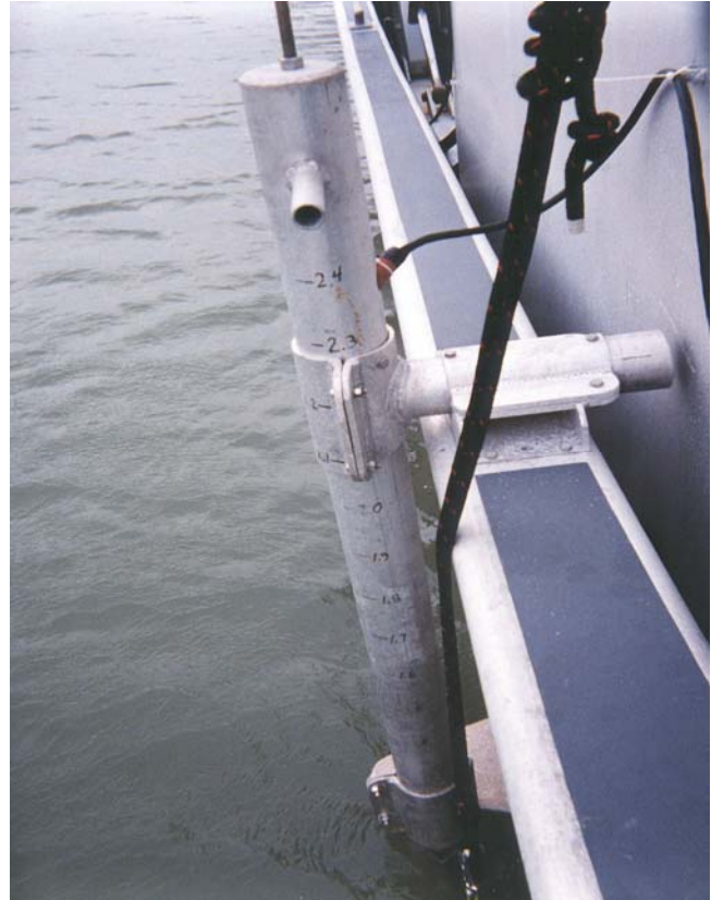
MULTIBEAM MOUNT WITH DRAFT MARKS
